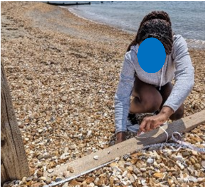
Figure 2: Measuring the groyne drop.
